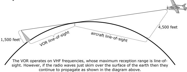
This means that you need to calculate the maximum line-of-sight distance from the VOR, and add to it the maximum line-of-sight distance from the aircraft (using the normal formula). This is shown below;
